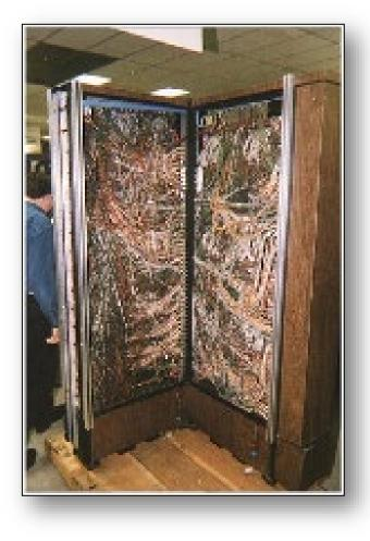
The microelectronics revolution allowed the amount of handcrafted wiring seen on the left to be mass-produced as an integrated circuit the size of your thumbnail.
